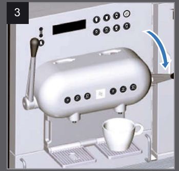
Pull down lever to the lowest position.
