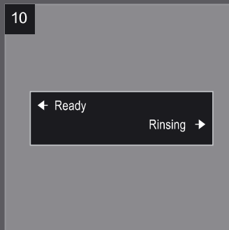
Automatic internal rinsing: An approx. 3 sec. internal rinsing of the milk system will begin immediately after each milk-based beverage preparation.
